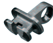
Built-in hinge: machining from wire, material CuNi18Zn20, 20 pieces/min. on NAM-8 (complete machining)
