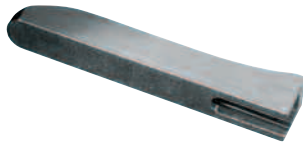
Complete machining: material CuNi18Zn20, 20 pieces/min. on NAM-10
