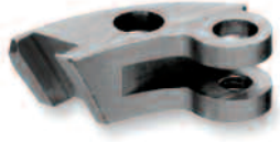
Curved hinge: complete machining CuNi18Zn20, 18 pieces/min. on NAM-8 (complete machining)
