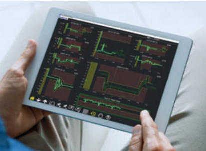
Mikron's miTool tool-monitoring system
