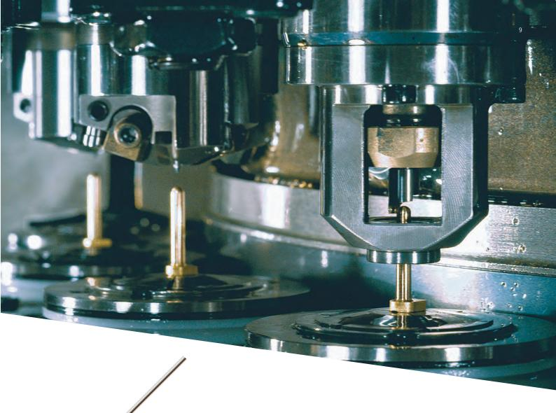
Mikron Multistar can be equipped with an advanced bushing guide systems that hold the part near the cutting tool during the turning operations, assuring high precision, no vibrations, and perfect surface finish for very challenging Diameter/Length ratio (70xD); example Ø 0.5mm length 36mm
