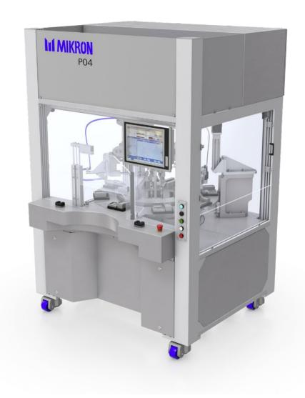
The Mikron P04 assembly system is based on standard building blocks from Mikron's proven platform library. The machine base version uses a central cam shaft to control working units for all primary motions.
