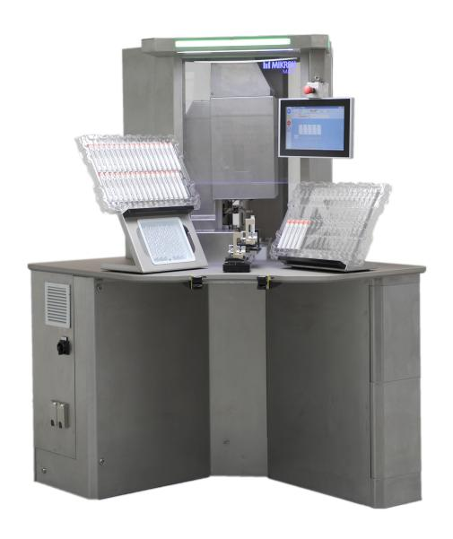
Mikron MAIA is a low volume assembly and test system to produce single or multiple variants of pen, auto-injectors or safety syringes.
